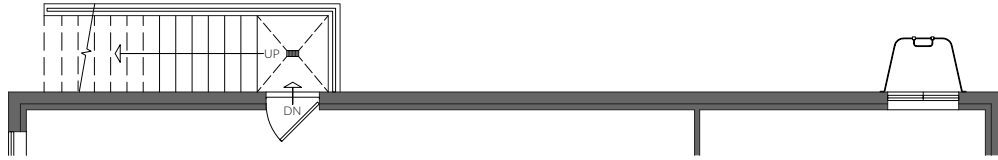
BASEMENT WITH OPT. WELLED EXIT "A"
